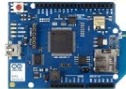
Arduino XBee Shield
